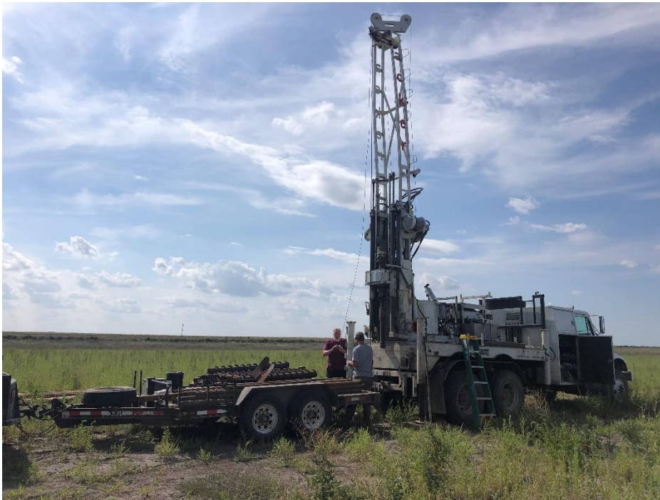
Hollow-stem auger w/ wireline splitspoon sampler
