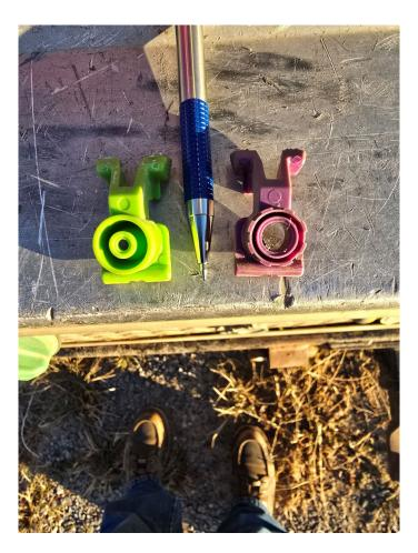
At 6psi this orifice will flow 6 gallons per minute. At 15 psi this orifice will flow 9.5 gallons per minute. This is 63% of designed flow.
