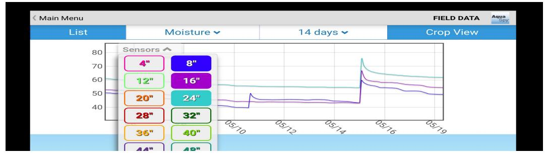
This picture is taken from the same probe as the previous one. The reading is broken down to a two week window, and only three of the sensors are turned on so that a specific range can be analyzed. The first bump on 5/11 shows a .70" irrigation pass that soaked in to a soil depth of 8-16" as expected. The second bump shows a 1.3" rainfall event that soaked in to a soil depth of 24", you can then see the moisture stepping down as the plants use the moisture in the top 8-16" soil zones.
