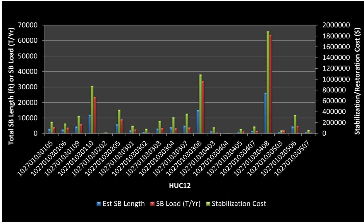
Figure 10: John Redmond Watershed Streambank Erosion Assessment Graph by HUC12
