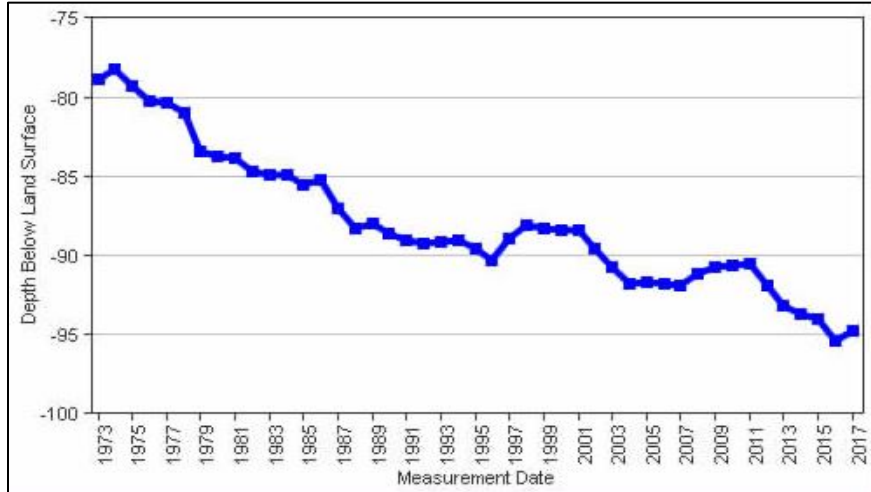
Figure 11: Hydrograph showing the decline of the Ogallala Aquifer through time, with well measurements near Dighton in Lane County
