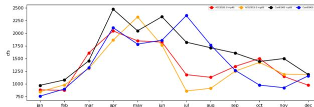
**Fig. 6** - Projected average monthly stream flow for USGS gage 06916600 under rcp45 and rcp85 climate scenarios for climate models ACCESS1-0 and CanESM2
