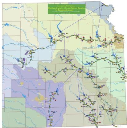
**Fig. 1** - A schematic of the KWO model used to allocate water in the state of Kansas. The water balance model incorporates six river basins, 21 reservoirs (16 are federal reservoirs), 51 inflows and 163 sources of consumptive use.
