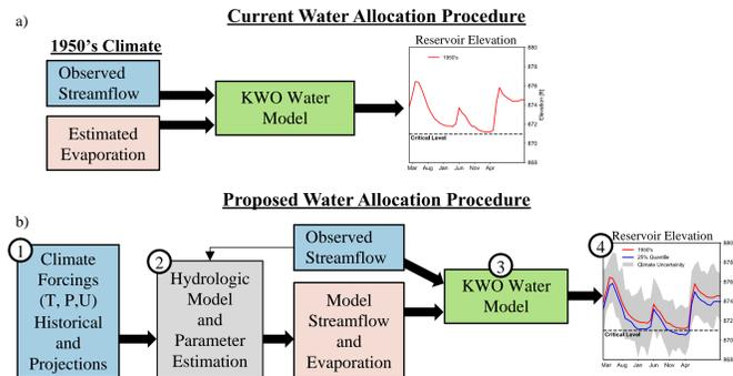
**Fig. 2** - a) The current practice at KWO is to use the model based on streamflow and evaporation estimated during the 1950's drought. b) The new water allocation procedure will include climate uncertainty into the water allocation procedure in Kansas by utilizing CMIP5 projections from 34 different models downscaled to 1/16<sup>th</sup> degree.
