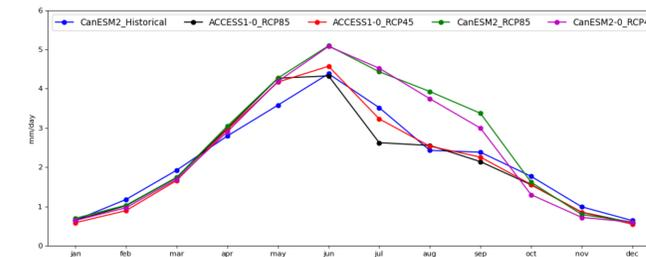
**Fig. 8** - Evapotranspiration from the modeled historical period and the RCP45 and RCP85 climate scenarios from the ACCESS1-0 and CanESM2 climate models for USGS gage 06916600.
