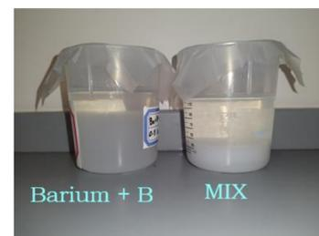
Solution chemistry also affected coagulant settling, and thereby Boron removals with individual cation solutions producing fluffy non-settling solids but the DGC composition had a powdery quick settling solid mass under same conditions.
