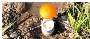
Fig 6: STIC logger deployed in the field, summer 2021
